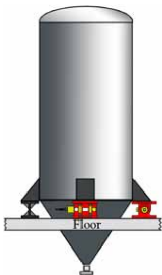
Low-accuracy, storage silo partially supported by KIS Weigh Modules.
